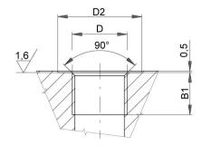
Standard fitting dimensions are used for connecting ports P, T, A, B of the manifold. It is recommended to provide O-ring sealing to all pipe or hydraulic hose fittings.
