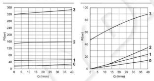
**0** = VMP10.0.. - **1** = VMP10.1.. - **2** = VMP10.2.. - **3** = VMP10.3.. Fluid used: mineral based oil with viscosity 46 mm<sup>2</sup>/s at 40°C.
