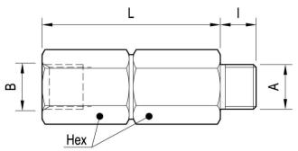
The valve is only available with G 1/4 ports, with different size restriction orifices, as indicated by the table of orifices.
